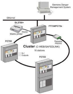
Using a fiber-optic Backbone (C-WEB/LAN) up to 14 of the above mentioned clusters (with up to 16 stations each) can be networked. The entire network may contain up to 64 stations.
