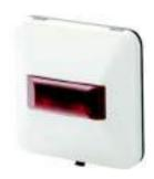
The alarm indicator is connected in parallel to automatic fire detectors in order to indicate quickly the source of an alarm signal from detectors that are not easily accessible or visible. The alarm indicator lights up as soon as a connected fire detector gives an alarm.
