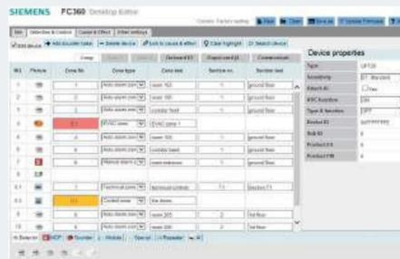
The FC360 configuration tool is simple to understand and use. The connected devices are listed in a table in their order of wiring, allowing the user to easily visualize the devices as installed. Outputs and sounders can be assigned into one of 16 control or evacuation zones and an appropriate description text (e.g., "door release") can be added for more clarity.
