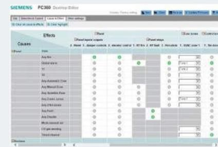
Most systems require all alarming devices and control outputs to operate with any fire. This operation is available by default. Where more complex controls are required, the FC360's unique cause-and-effect matrix makes any required changes easy and logical.
