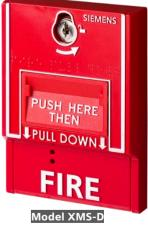
The XMS-S & XMS-M manual station front cover has a recess pocket to pull down and locks in position after the alarm is initiated. The XMS-D, XMS-DA & XMS-2S manual stations have an additional lever labeled "PUSH HERE THEN" to get access to the front cover pocket to initiate the alarm.
